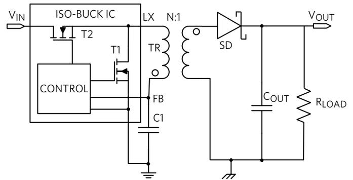
Figure 4. Iso-Buck converter
