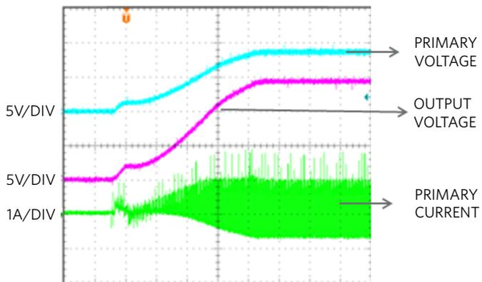
Figure 7. MAX17681 Iso-Buck monotonic startup
