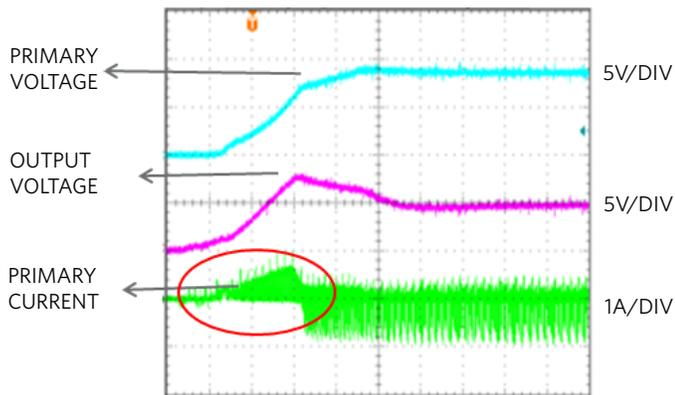
Figure 6. Standard buck non-monotonicity in Iso-Buck mode
