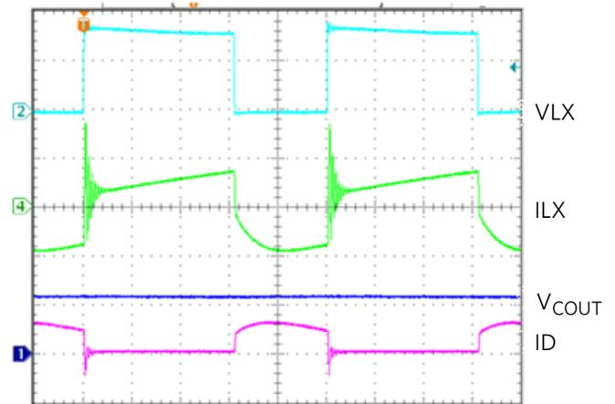
CH2:LX VOLTAGE, CH4:LX CURRENT, CH3:SECONDARY CURRENT, CH1:V<sub>OUT</sub>
